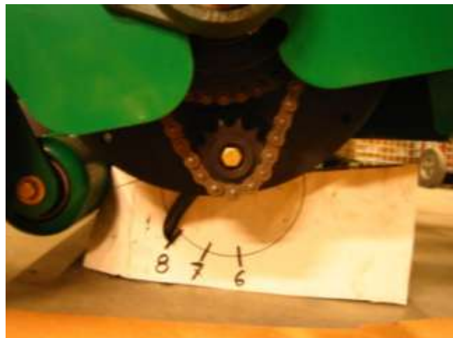
Rotate the rotor to make sure each shaft aligns to 8 o'clock position at the bottom of rotation
