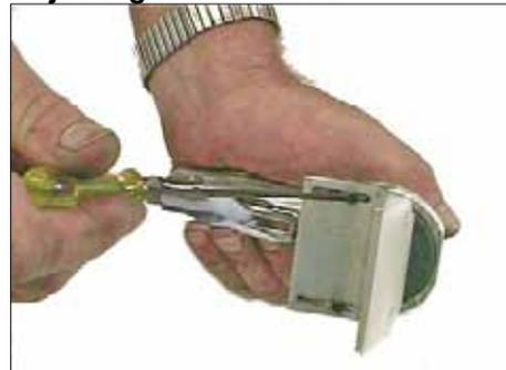
You can adjust the height of the guide by loosening the two socket head screws and sliding the guide up or down. If the front facer bogs down, you should adjust the fence up so that less of the disc surface contacts the bed knife. You can also check your air pressure or use shorter air lines.
