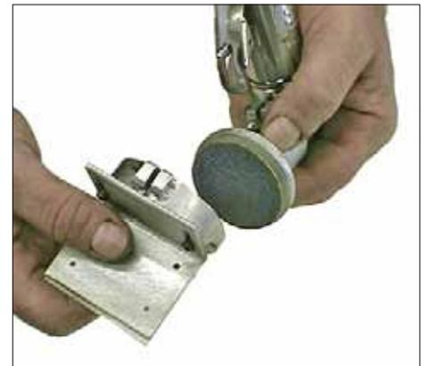
Remove the guide assembly. You may need to loosen one of the guide adjusting screws for the clamp to loosen.
