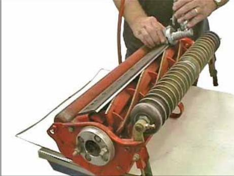
Place the nylon pad on the bottom of the bed knife just in from the end and hold the grinding disc away from the bed knife edge.
