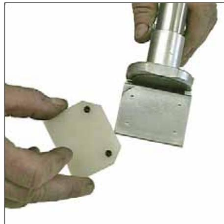
Remove the two socket head screws which secure the nylon pad and replace with the selected pad.
