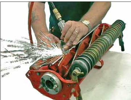
Pull the front facer back to the beginning of the bed knife then push it to the end of the bed knife. Repeat as necessary.
