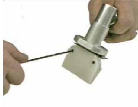
The front facer comes with four angle pads; 0°, 5°, 10° and 15°, which can be mounted to give either a positive or negative relief angle. Refer to your mowers manual to determine which pad to use.
