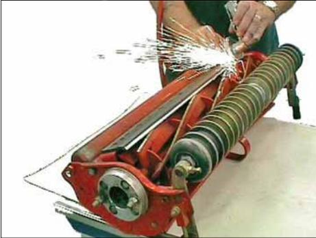
Pull the trigger of the front facer and push it against the bed knife.
